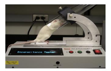
**Fig. 1.** Modification of the rodent incapacitance tester showing a rat in the correct resting position. The advantage of the tube is that it encourages the animal to stand with its weight directed onto the force plates.
